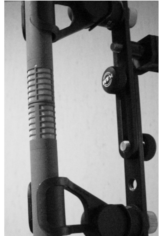
Two microphones (with lateral pickup) arranged for optimum coincidence in the horizontal plane.
