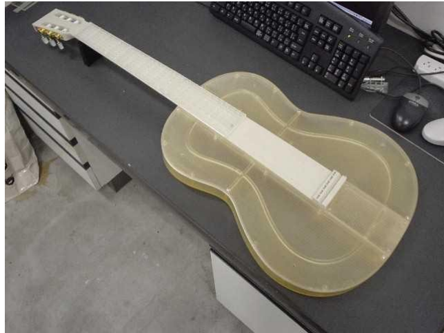
Figure 2. Photo-reflector based fingering capture system.
