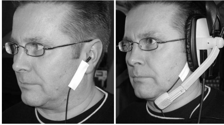
Figure 1: The miniature microphone was positioned at the entrance of an open ear canal for MIRE-recordings.
