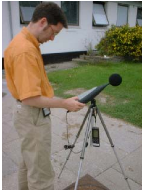
Figure 1. Using a GPS unit with a sound level meter.
