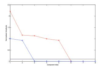
Figure 5: Normalized amplitude of the components estimated using the ARMA (square) and the HR (circle) focused analysis methods in the case of a test signal consisting of two closely spaced modes. Only the components with amplitude higher than the threshold (solid line) are considered.
