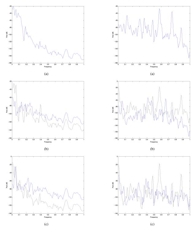
Figure 6: Normalized Power Spectral Density of a guitar sound (a) and the corresponding estimated excitation using a HR broadband analysis only (dashed line) and in solid line, a Fourier broadband analysis followed by, respectively, the ARMA focused analysis (b), and the HR focused analysis (c).
