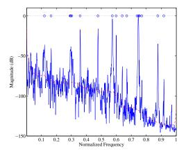
Figure 3: Frequency Histogram (solid line) used to identify the modes. The median filtered version (dashed line) is removed prior to thresholding.
