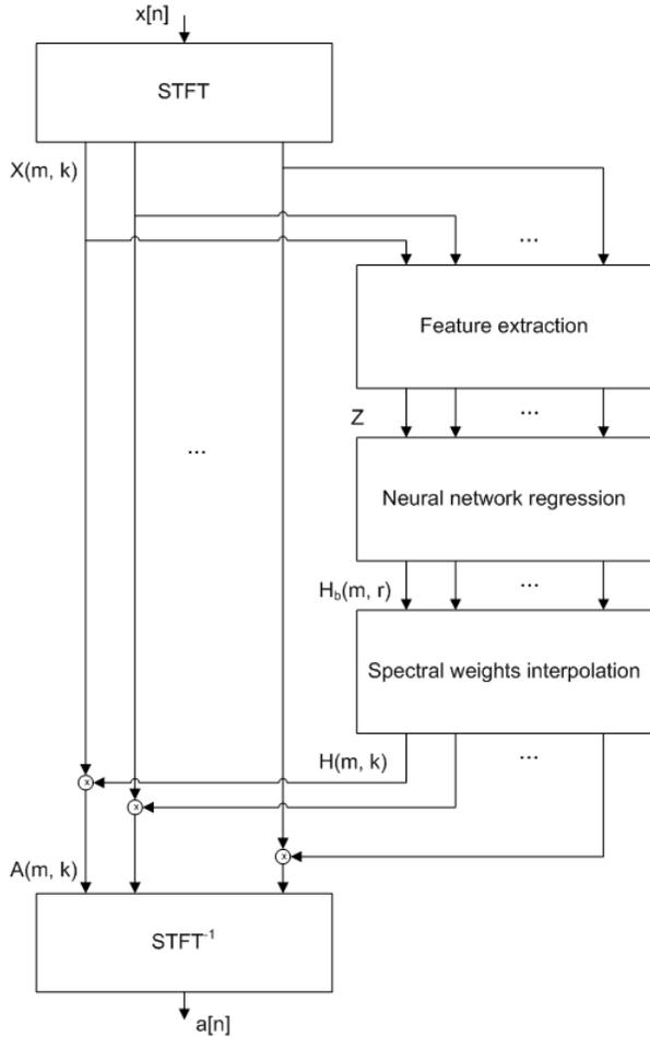
Figure 1: Block diagram of the ambient extraction processing.
