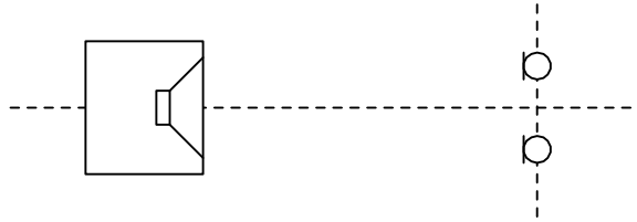
Figure 3.7: Calibration scheme. The reference microphone and the subject are symmetrically positioned aside the sound source perpendicular. The distance from the sound source is adequate for far field conditions.
