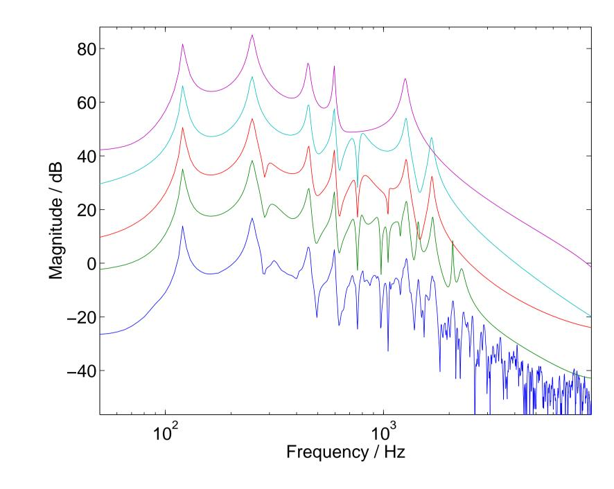
The warped BU-method finds the five prominent resonances at filter order 10, in contrast to the unwarped design, where the required order is about 100! Finally, we demonstrate that good fit to the five prominent resonances of the 10th order Kautz filter means also good match in the time-domain to the measured response:
