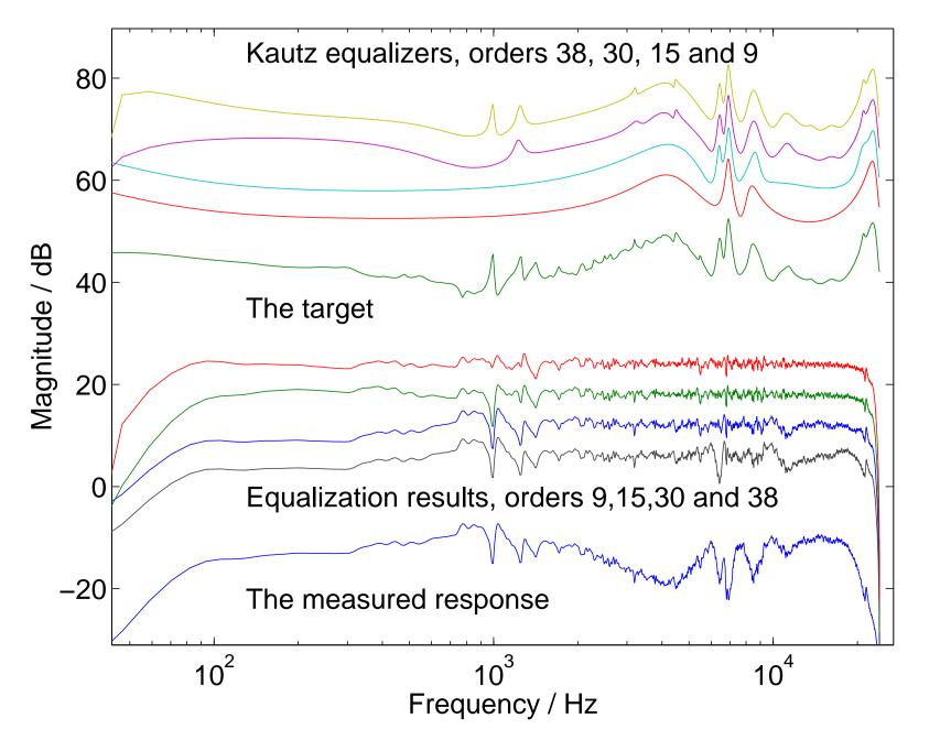
To improve the modeling at 1 kHz, we add 3–4 manually tuned pole pairs to the BU-pole sets, omitting some undesired poles, producing
