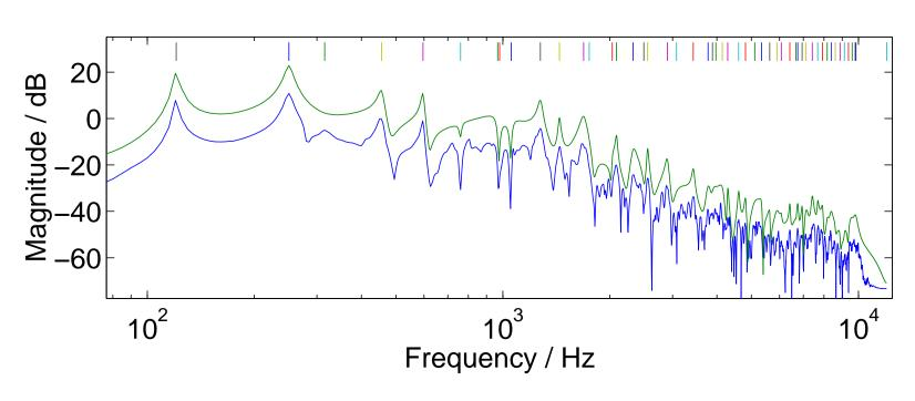
Lines indicate pole pair positions. Especially in this case of a target response dominated by the low-frequency part, we may compose very low order Kautz
