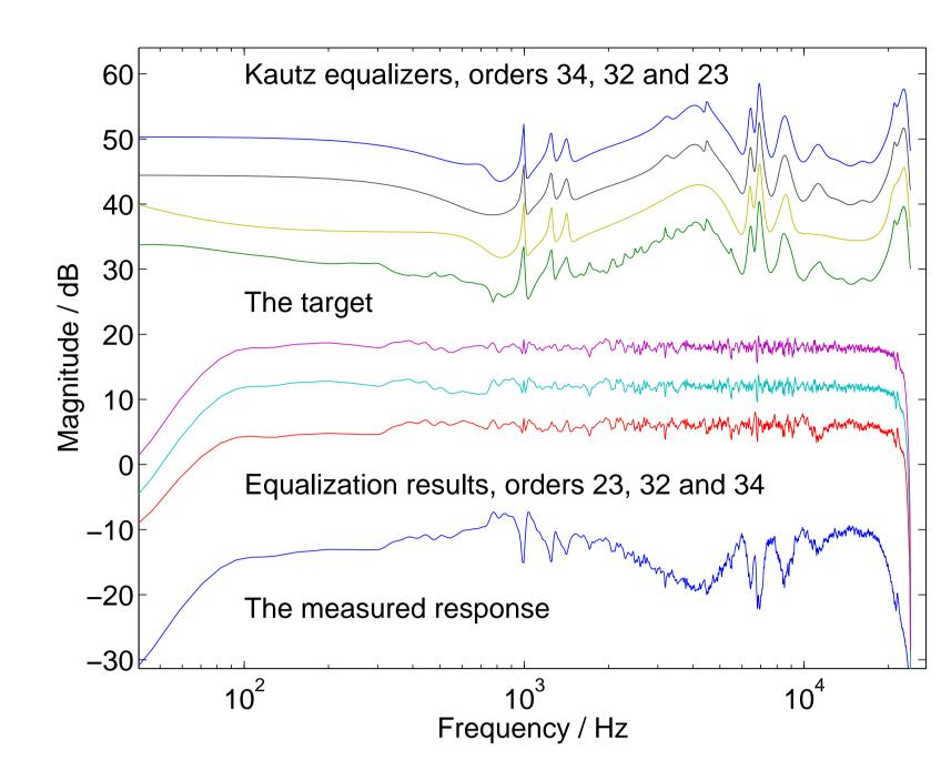
We may also tune all the poles manually, e.g., with 10 distinct pole pairs, chosen and tuned to fit the magnitude response:
